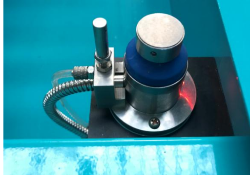
Tool Sensor Automatic tool sensor with air blower
