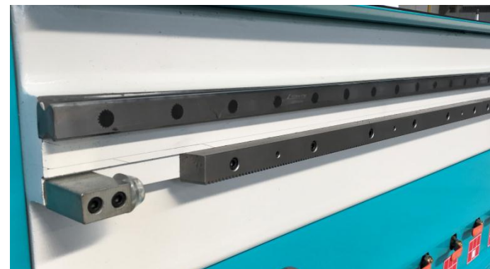
Y axis Transmission 1.25M Rack & Pinion; 25mm Square Guide rail; Block
